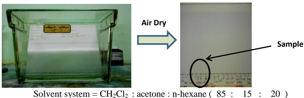
Figure 2 Extraction of aflatoxin by TLC
