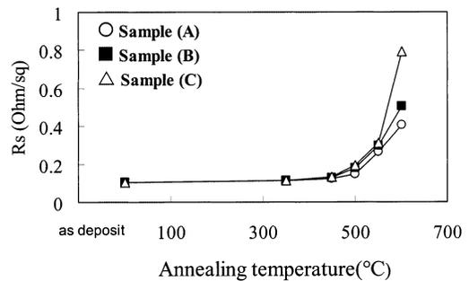
Fig. 3. Variation of sheet resistances of Cu/TaN/SiO<sub>2</sub>/Si multilayer structures as a function of annealing temperatures.
