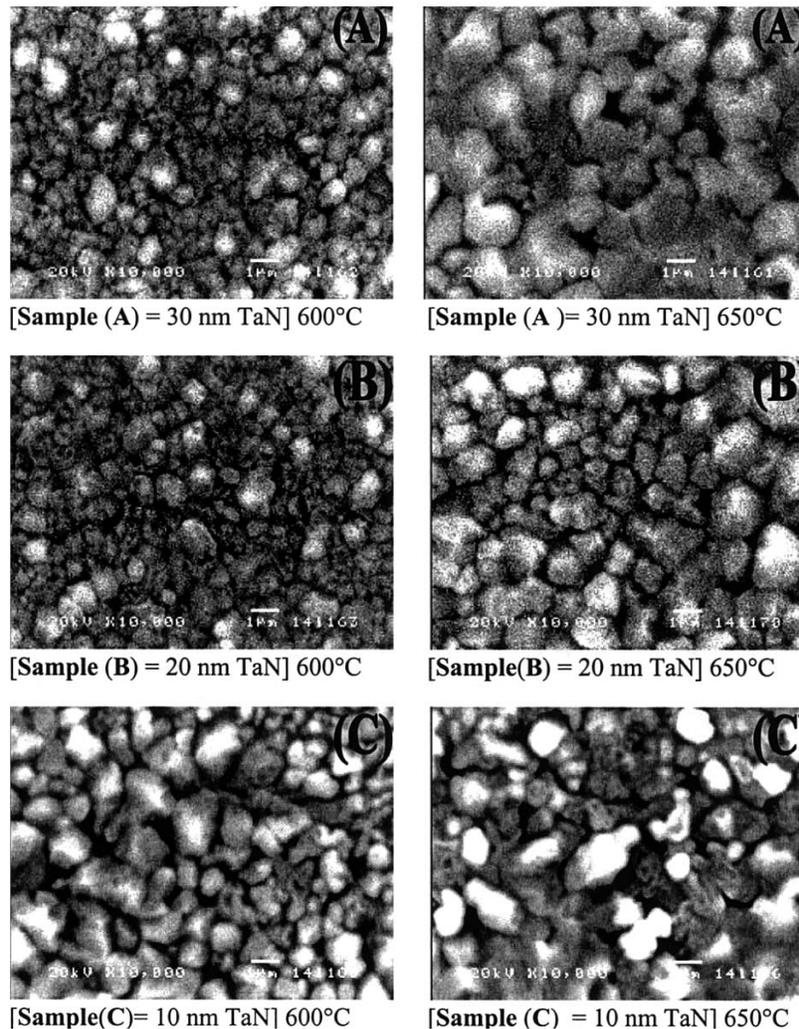
Fig. 10. SEM micrograph of the Cu/TaN/SiO<sub>2</sub>/Si multilayer structures after annealing at 600 and 650°C.
