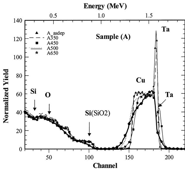
Fig. 7. 2 MeV  $\text{He}^+$  RBS spectra of Cu/TaN(30 nm)/ $\text{SiO}_2$ /Si multilayer structure annealed at various temperatures.
