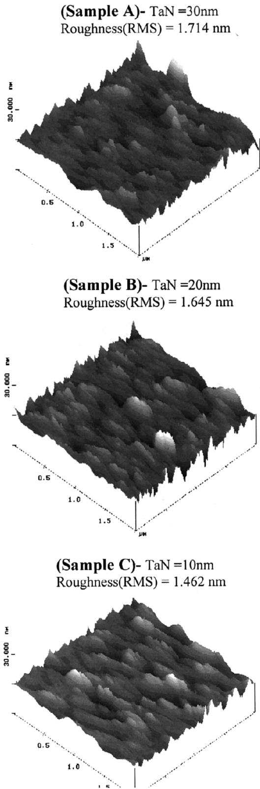
Fig. 2. AFM measurement results of the as-deposited TaN samples with different thicknesses.
