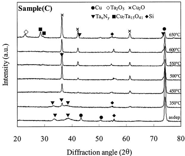
Fig. 6. XRD patterns of the Cu/TaN(10 nm)/SiO<sub>2</sub>/Si multilayer structure annealed at various temperatures for 35 min in N<sub>2</sub> ambient.
