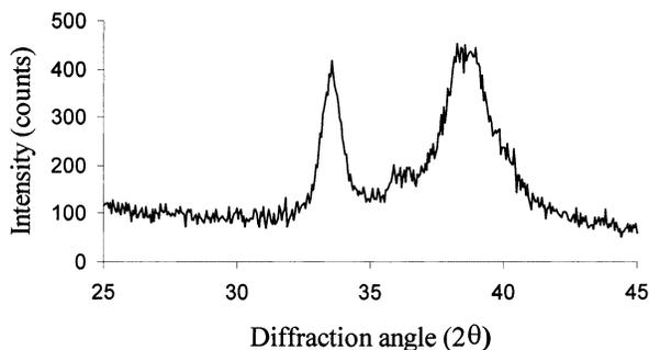
Fig. 1. XRD pattern of as-deposited TaN showing amorphous and/or nanocrystalline structure.
