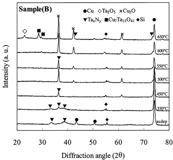
Fig. 5. XRD patterns of the Cu/TaN(20 nm)/SiO<sub>2</sub>/Si multilayer structure annealed at various temperatures for 35 min in N<sub>2</sub> ambient.
