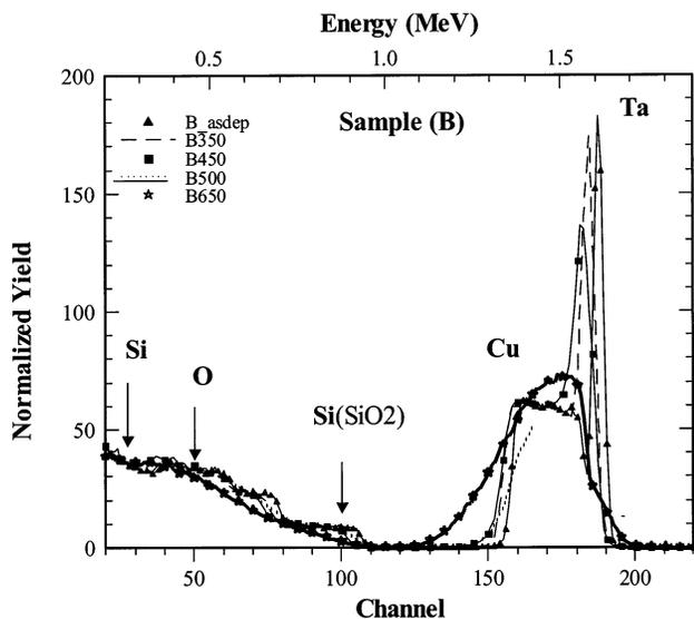
Fig. 8. 2 MeV  $\text{He}^+$  RBS spectra of Cu/TaN(20 nm)/ $\text{SiO}_2$ /Si multilayer structure annealed at various temperatures.
