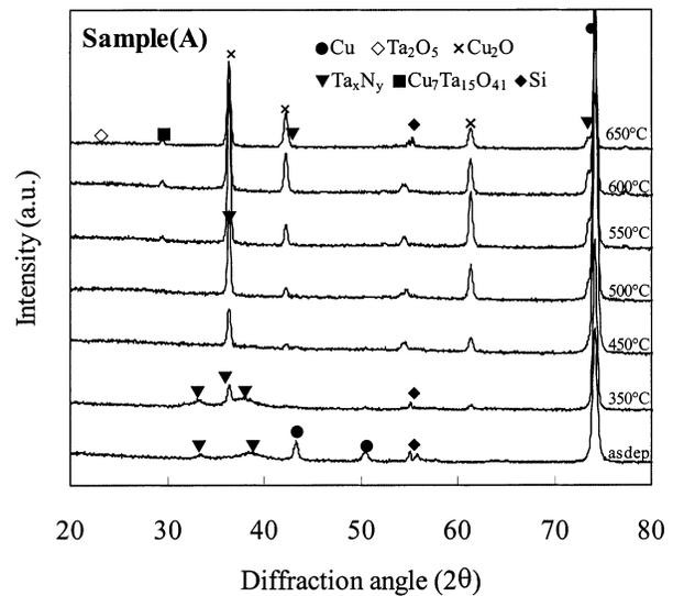
Fig. 4. XRD patterns of the Cu/TaN (30 nm)/SiO<sub>2</sub>/Si multilayer structure annealed at various temperatures for 35 min in N<sub>2</sub> ambient.
