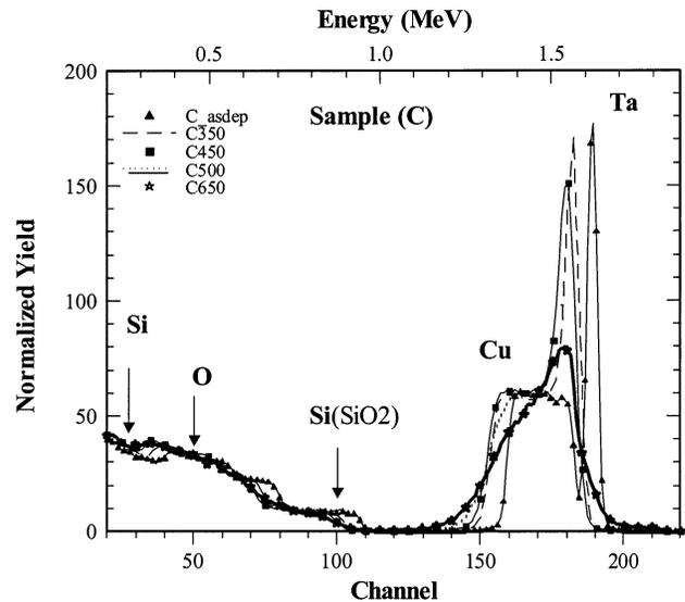
Fig. 9. 2 MeV  $\text{He}^+$  RBS spectra of Cu/TaN(10 nm)/ $\text{SiO}_2$ /Si multilayer structure annealed at various temperatures.
