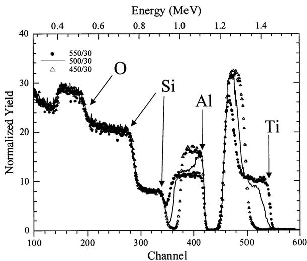
Fig. 6. RBS spectra of Al-0.5 wt.% Cu/Ti/SiO<sub>2</sub>/Si structure after annealing at 450, 500 and 550°C for 30 min in Ar ambient.
