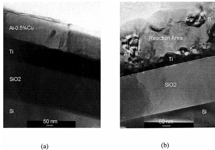
Fig. 3. Cross-section morphologies (TEM) of the Al–0.5 wt.% Cu/Ti/SiO<sub>2</sub>/Si structure (a) as deposited, (b) annealed at 600°C.
