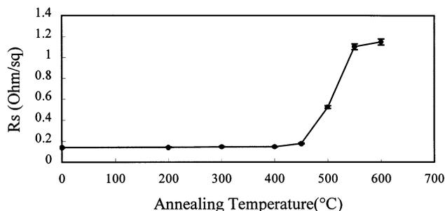
Fig. 1. Variation of the sheet resistance in Al–0.5 wt.% Cu/Ti/SiO<sub>2</sub>/Si structure as a function of annealing temperature.
