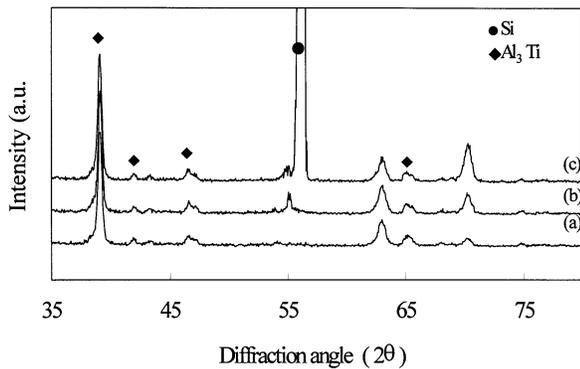
Fig. 5. The XRD spectra of Al-0.5 wt.% Cu/Ti/SiO<sub>2</sub>/Si structure annealed at 500°C for 30 min in Ar ambient with different grazing incident angles (a) 0.5°, (b) 1.0° and (c) 1.5°.
