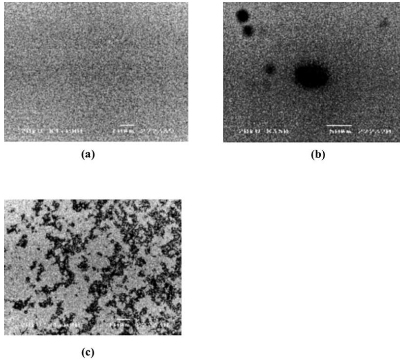
Fig. 2. SEM surface morphologies of the Al–0.5 wt.% Cu/Ti/SiO<sub>2</sub>/Si structure (a) as deposited (b) annealed at 500, (c) annealed at 550°C.
