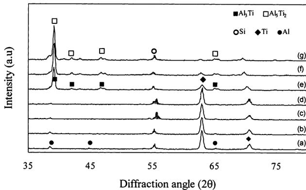
Fig. 4. The XRD spectra of samples (a) as deposited, (b) annealed at 300°C, (c) annealed at 400°C, (d) annealed at 450°C, (e) annealed at 500°C, (f) annealed at 550°C, (g) annealed at 600°C.
