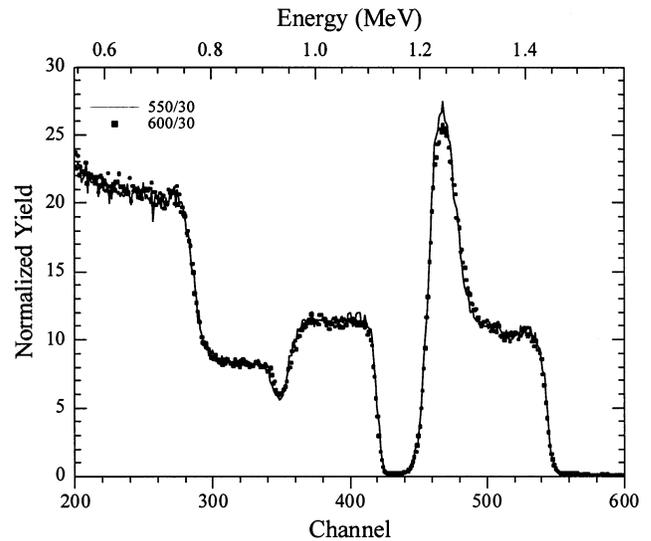
Fig. 7. RBS spectra of Al-0.5 wt.% Cu/Ti/SiO<sub>2</sub>/Si structure after annealing at 550 and 600°C for 30 min in Ar ambient.
