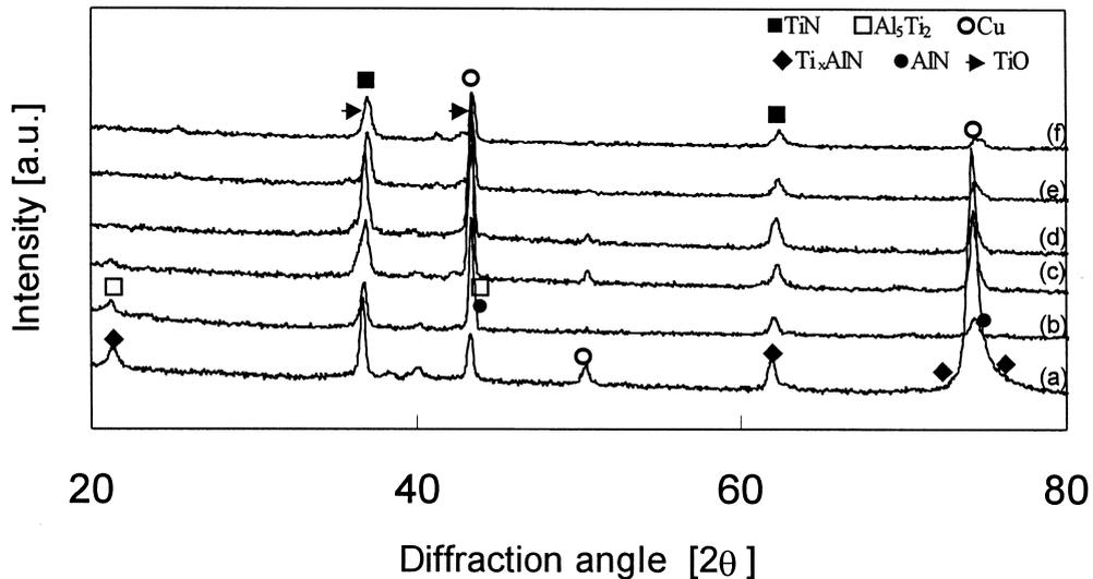
Fig. 2. XRD spectra of the Cu/Ti<sub>x</sub>Al<sub>y</sub>N<sub>z</sub>/SiO<sub>2</sub>/Si structure before and after annealing at (a) 550°C, (b) 650°C, (c) 750°C, (d) 850°C, and (e) 950°C.
