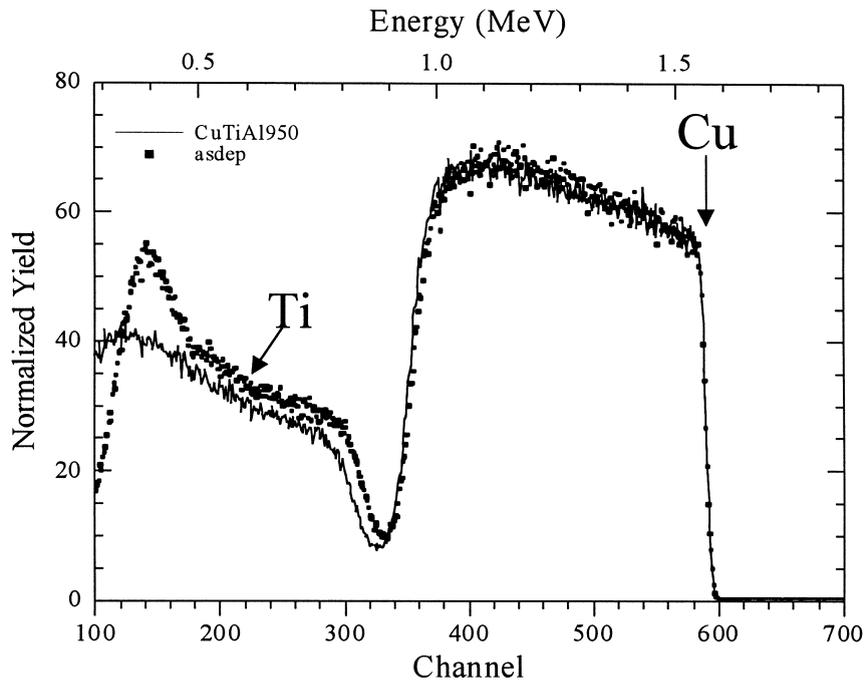
Fig. 3. 2 MeV He<sup>+</sup> RBS spectra of the Cu/Ti<sub>x</sub>Al<sub>y</sub>N<sub>z</sub>/SiO<sub>2</sub>/Si structure before and after annealing at 950°C.
