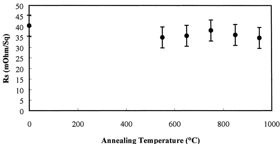
Fig. 1. Variation of sheet resistance in Cu/Ti<sub>x</sub>Al<sub>y</sub>N<sub>z</sub>/SiO<sub>2</sub>/Si structure as a function of annealing temperature.
